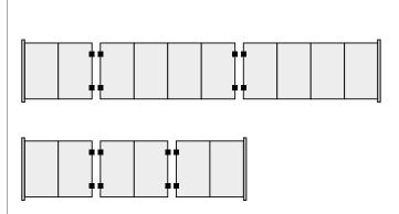
Installation spacers X (reveal is not adjustable) on the running and guide components permits door combinations on uninterrupted runner and guide profiles.
