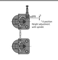
Note: installation and removal are only possible in 0-position, i.e. with 3 mm clearance
